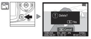
To delete the photograph currently displayed in the monitor, press 📆. A confirmation dialog will be displayed. Press in again to delete the image and return to playback. To exit without deleting the photograph, press **•**.
