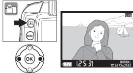
Additional photographs can be displayed by rotating the command dial or pressing the multi selector left or right. To view highlights or additional photo information about the current photograph, press the nuiti selector up or down. See page 73 of the User's Manual for details. To end playback and return to shooting mode, press the shutter-release button halfway.
