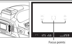
Slide the diopter adjustment control up and down until the focus points are in sharp focus. When operating the diopter adjustment control with your eye to the viewfinder, be careful not to put your fingers or fingernails in your eye.
