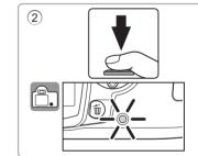
Smoothly press the shutter-release button the rest of the way down to release the shutter and record the photograph. The memory card access lamp will light. Do not open battery-chamber cover or the memory card slot cover until the memory card access lamp has gone out and recording is complete.
